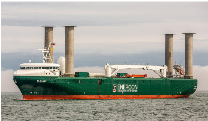
The E-Ship 1 is a Flettner ship: four large rotorsails that rise from its deck are rotated via a mechanical linkage to the ship's propellers. Alan Jamieson from Aberdeen, Scotland, CC BY 2.0 < https://creativecommons.org/licenses/by/2.0/ >, via Wikimedia Commons
